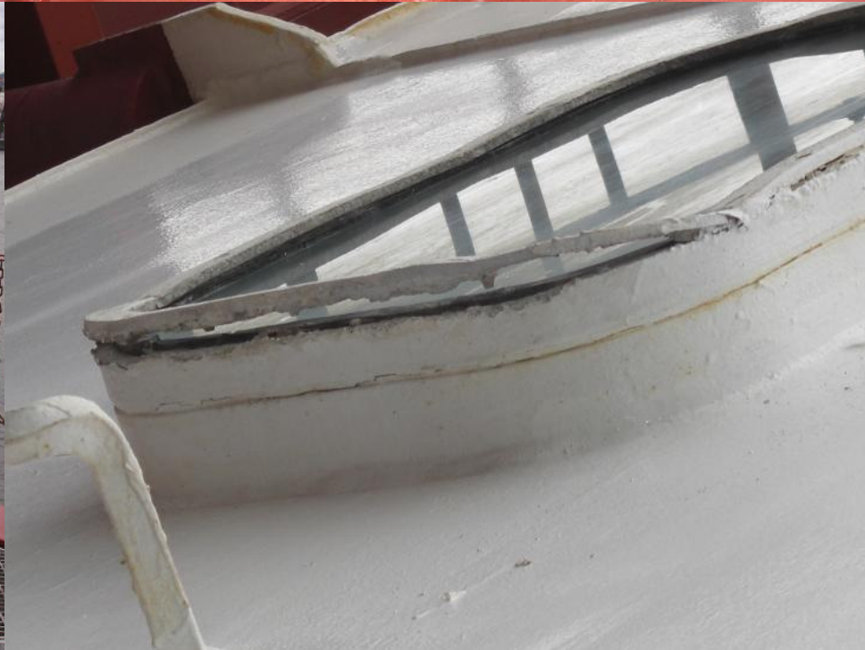
MV Laura Schulte: insufficient working safety on deck, watertight flaps not properly closable, window frames wasted
